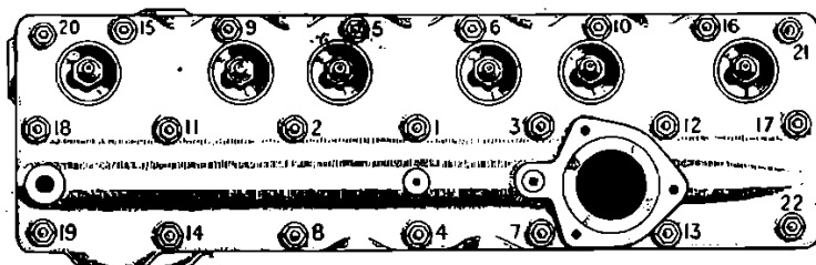
Figure 4. Cylinder Head (Showing order of tightening head nuts)
